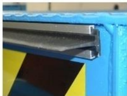
Side-seal Seal at the edge of the leveller
